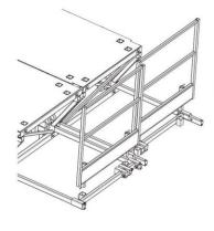
Install every bottom outrigger and secure in place with provided 5/8" bolts.
