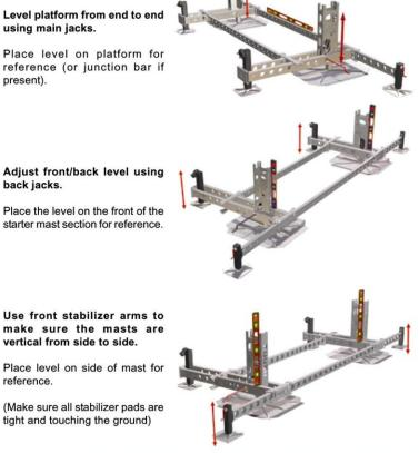
Page (28) CHAPTER 3: Positionning & levelling the platform
