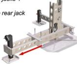
(7) Set unit in place along wall and set back 26" to 28" from finished wall. This will allow a 3 planks set-up
