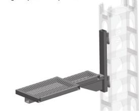
To install the rest platform, simply slide it in the mast rung, on the wall side of mast, as shown on the illustration.
