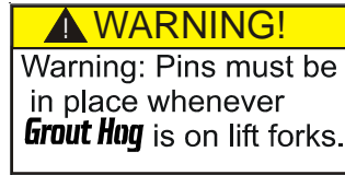
Pin Label: located on Fork Pockets
