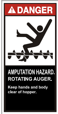
Amputation Label: located on back of hopper slightly left of center
